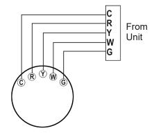
SINGLE STAGE HEATING & COOLING THERMOSTAT DIAGRAM
