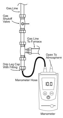
MEASURING INLET GAS PRESSURE (ALT. METHOD)
